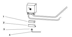
Mount the electronic box to the wall location using screw(1) and hex key provided (2).
